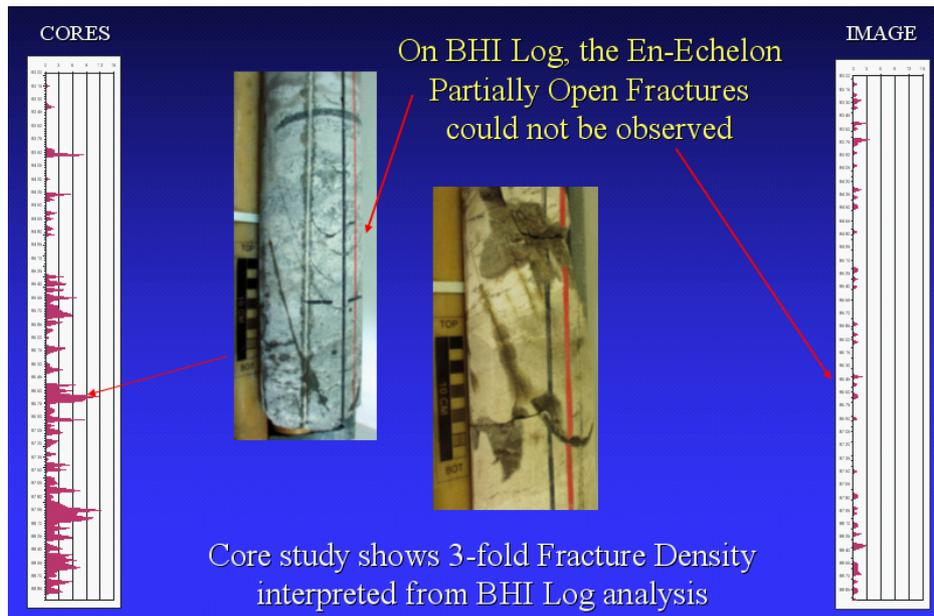
Figure 8 Many 'En Echelon' natural fractures did not appear on BHI log, leading to unrepresentative fracture density.
