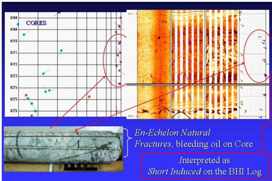
Figure 7 Many Natural 'En Echelon' fractures on cores reported as short induced fractures on BHI log.
