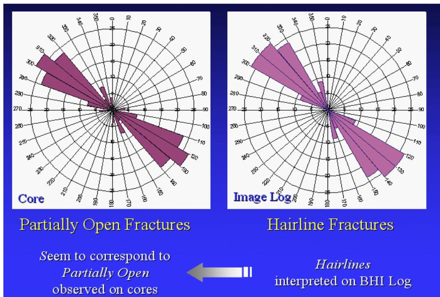
Figure 4 Partially Open Fractures Interpreted as Hairline Fractures on BHI log
