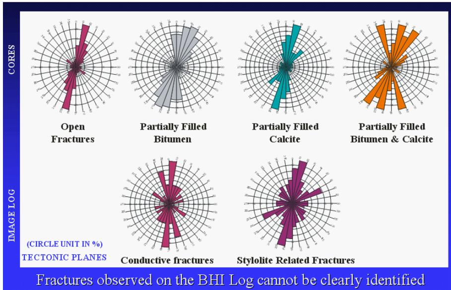
Figure 6 Core strike rose diagrams showing open fractures, partially open fractures and filling material. BHI strike rose diagrams showing only conductive and stylolite related fractures.
