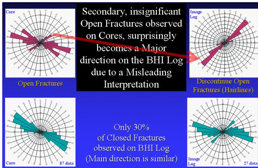
Figure 12 BHI interpretation could lead to a wrongful view of fracture density and fractures direction of the different fracture families.
