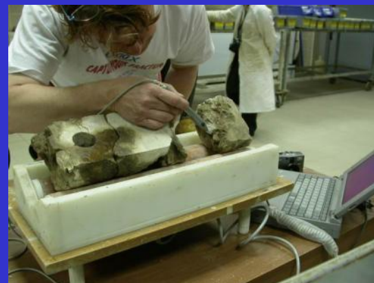
Possible to analyse slabbed cores and small core pieces
