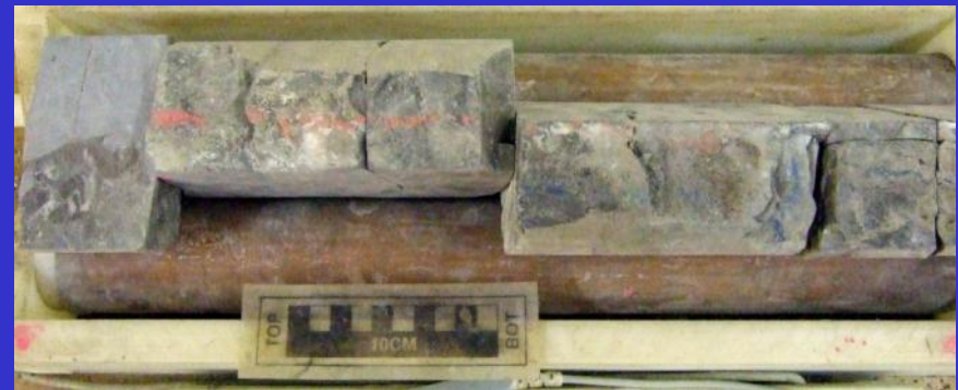
Examples of erratic slabbing
